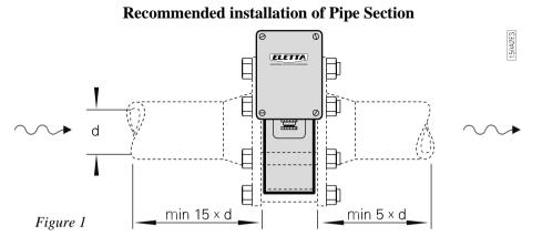
The reason for this procedure is to achieve a stable flow profile inside the pipe and by doing so, get a true reading. Please be aware of the fact that it is practically impossible to predict when the flow is stable after disturbances in the piping, so this must serve as a
