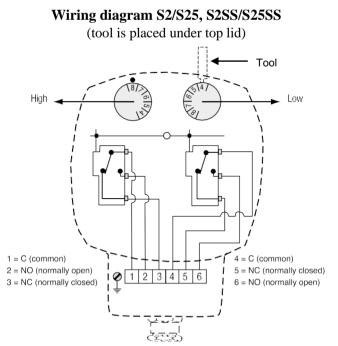
The wiring diagram shows the switching function when the flow is zero or below the lower setpoint.
